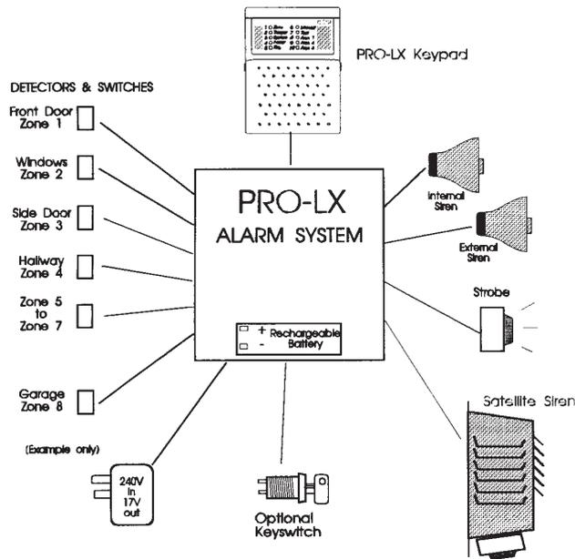
What you will see and use is the PRO-LX Keypad which is set up for you to control the Control Panel and view indicators to find out what is happening. In addition to the keypad may be a key switch or other controls such as push buttons. Your installer will explain the function of all such controls and you will also find them mentioned in the next two chapters.
