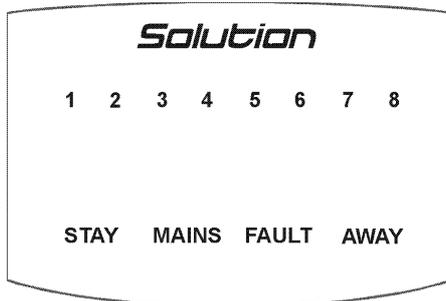
The codepad is the communications interface between you and your alarm system. It allows you to issue commands and offers both visual and audible indications that guide you through the general operation.
