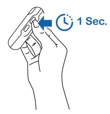
To turn on the device: press the CALL button for 1 second, all the LEDs will flash rapidly. The device can also be turned on automatically by charging via magnetic USB cable or put it into the docking station.
