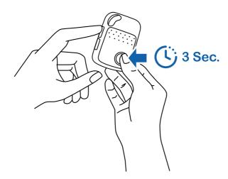
• To turn off the device: press and hold the side button and SOS button together for 3 seconds until the LEDs turn off.
