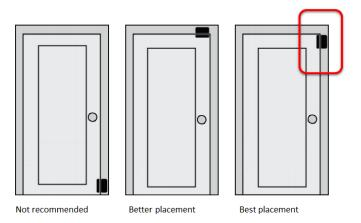
The sensors and magnet each have a slightly engraved line. This line denotes where the sensors align to function properly. If the sensor and magnet, when together/closed, do not line up correctly, the sensor will not report correctly. See Figure 2.
