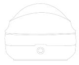
b. Gently slide a fingernail/fingertip into the slot and push the top casing of the sensor upward.(You can see the FCC label on the inside of sensor casing.)
