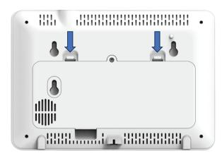
Lay the panel face down and remove the battery cover.
