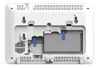
Plug the battery cable into the BATTERY port. Plug the power cable into the DC port.
